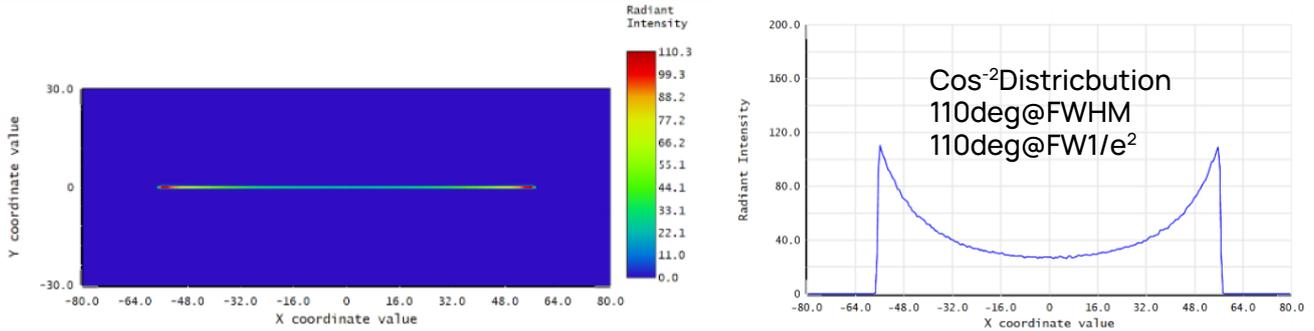
Angular Distribution Pattern (Left) and Angular Output Profile (Right)
