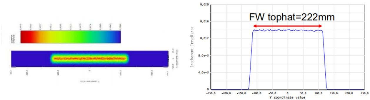
Spatial Distribution Pattern (Left) and Long Axis Spatial Output Profile (Right), 0.2 meter away from Diffuser
