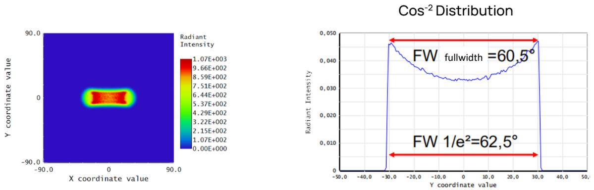
Angular Distribution Pattern (Left) and Angular Output Profile (Right)
