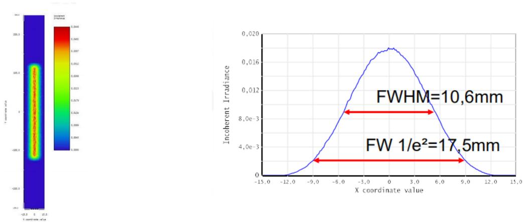
Spatial Distribution Pattern (Left) and Short Axis Spatial Output Profile (Right), 0.2 meters away from Diffuser
